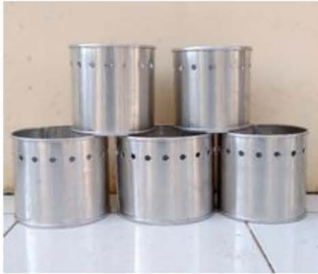
Figure 1. The shell of burning chamber
